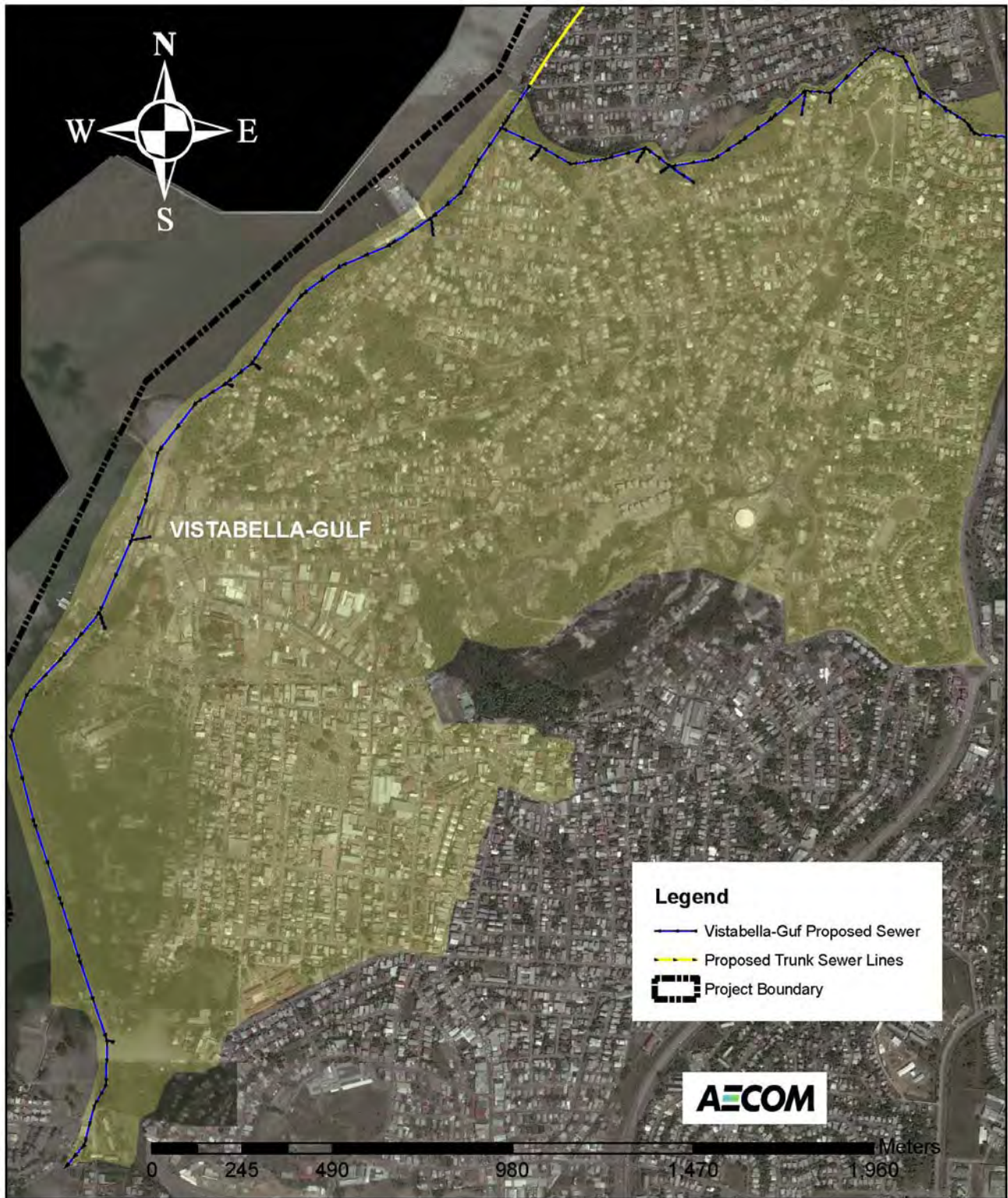
Figure 3-29 Vistabella-Gulf Subcatchment New Sewer Layout
