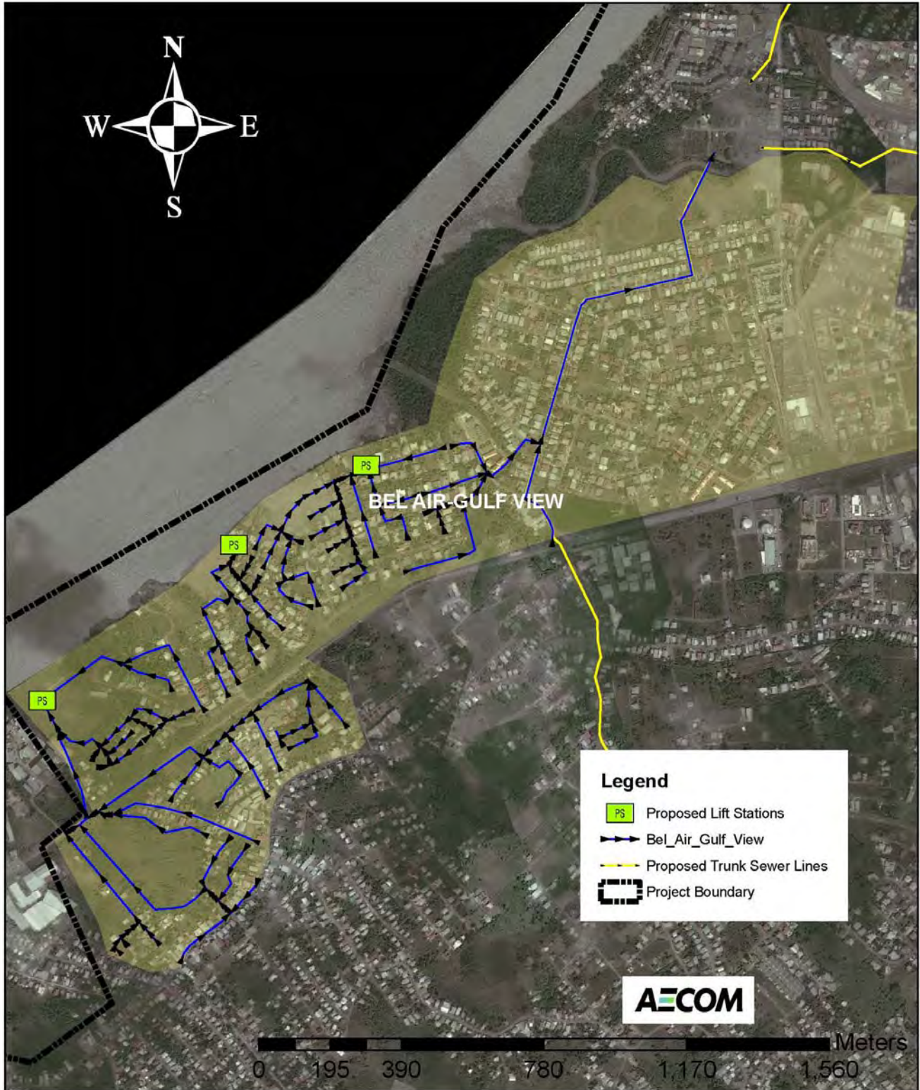
Figure 3-32 Bel Air-Gulf View Subcatchment New Sewer Layout
