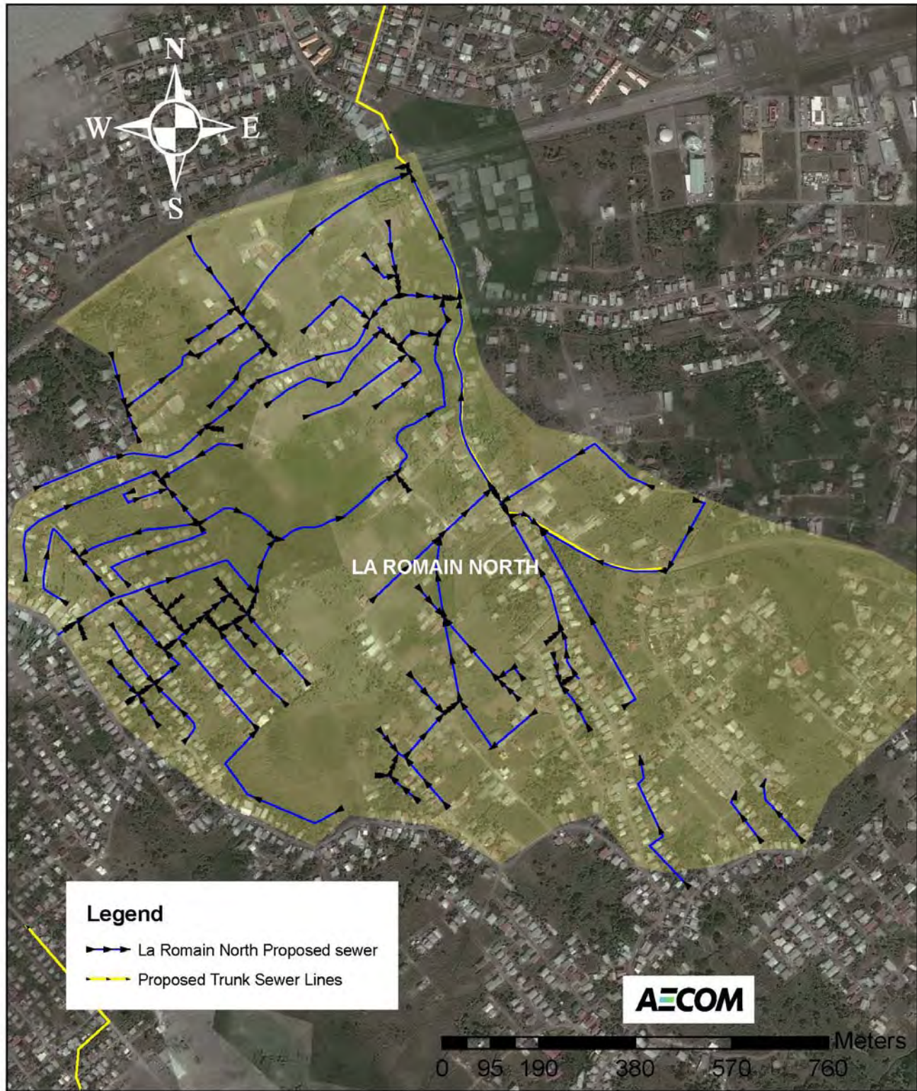
Figure 3-37 La Romain North Subcatchment New Sewer Layout
