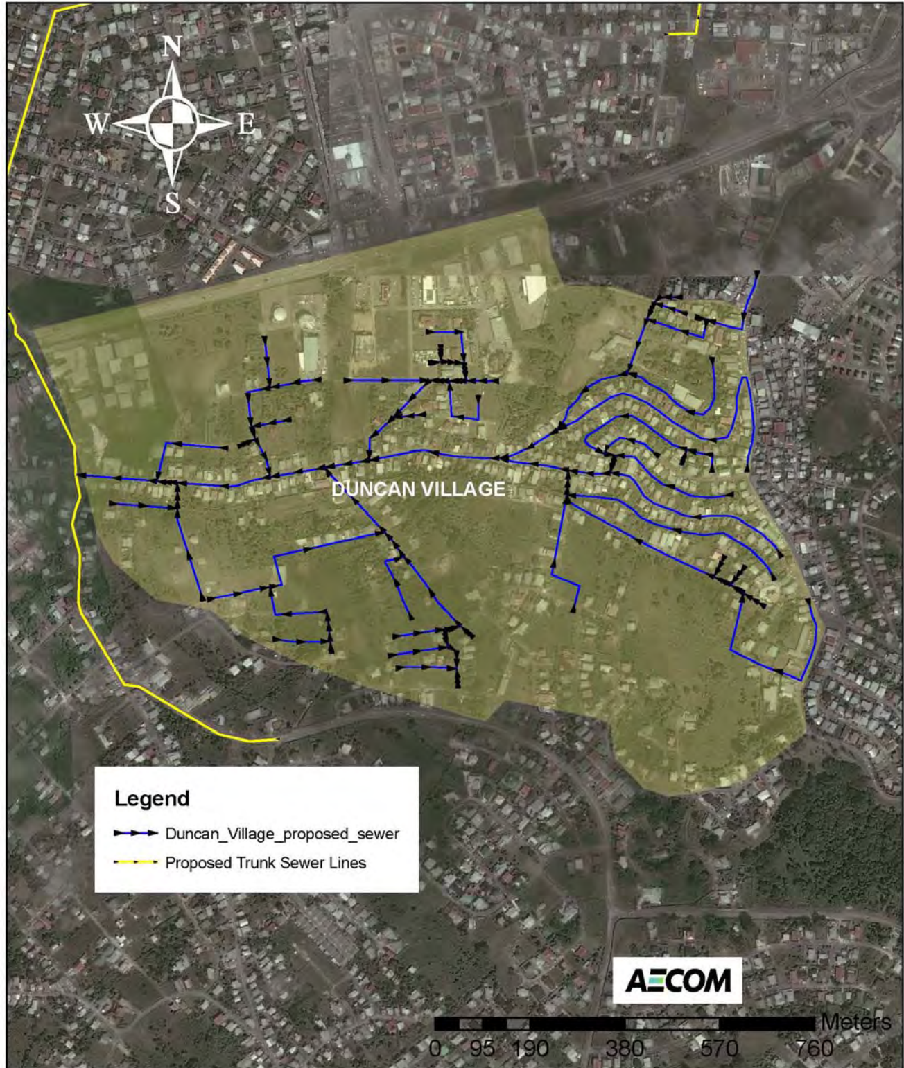
Figure 3-34 Duncan Village Subcatchment New Sewer Layout
