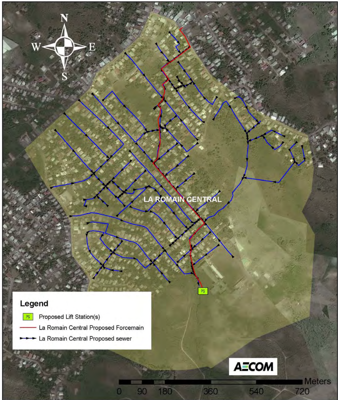
Figure 3-38 La Romain Central Subcatchment New Sewer Layout
